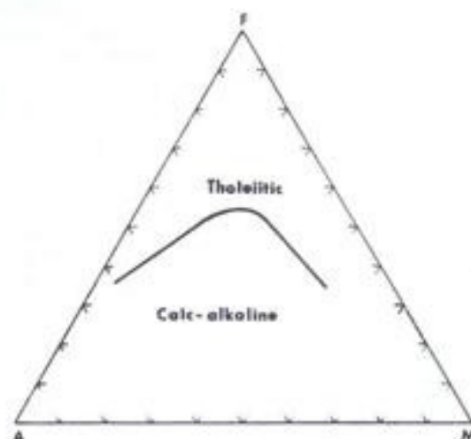
Figure 4-8 AFM plot showing line separating fields of tholeiitic and calc-alkaline rocks as proposed by Irvine and Baragar (1971). A = Na_2O + K_2O ; F = FeO + 0.8998Fe_2O_3 ; M = MgO , all in weight percent.
