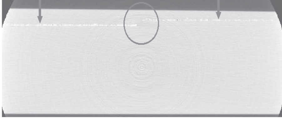
Figure 9.12 A CT-scan of a physical model with an interface between white rubber and Plexiglas. Traces of fine brass powder were added along the flat parts of the interface, as indicated by two arrows, to enhance its image. The circle highlights a gap in the interface without brass powder.
