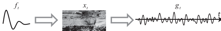
Figure 2.1 A source wavelet f_t traverses through the Earth x_t , producing a seismic trace g_t .
