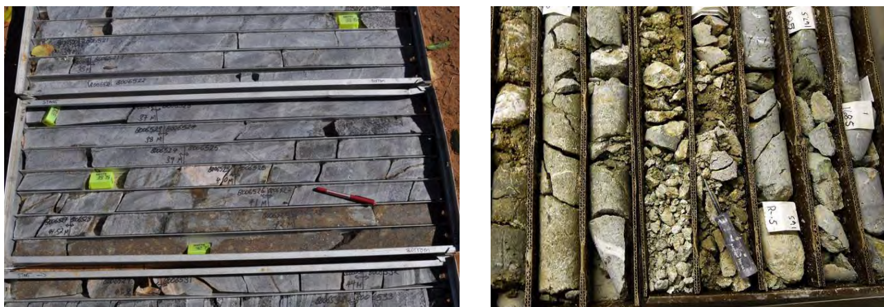
Figure 19.4: a) Fresh core with high core recovery in the mineralised zone, and b) highly weathered core difficult to log and sample in the mineralised zone
