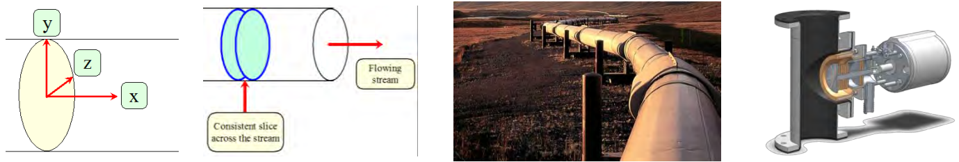
Figure 19.11: a) Increment delimitation in three dimensions (40) Pitard, F, 2009.), b) one dimensional sampling across a flowing stream (40) Pitard, F, 2009.), c) Canadian west-east oil pipeline, and d) an in-line stream sampler injector or thief sampler http://www.edart.co.za/
