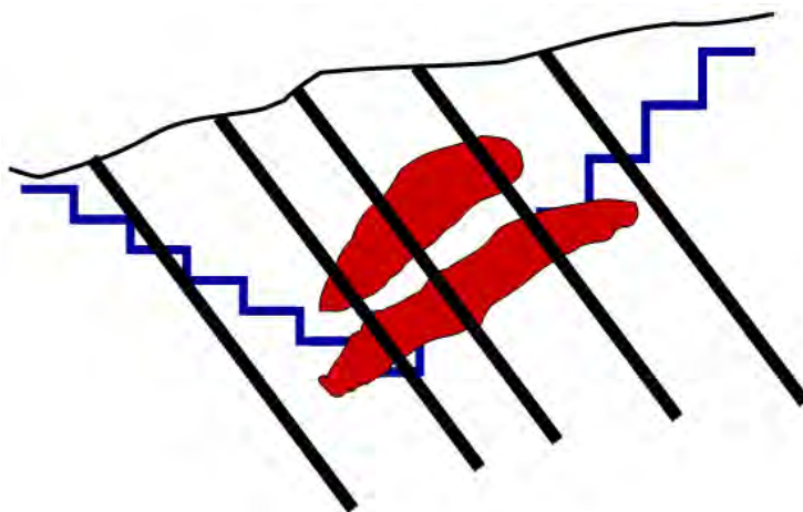
Figure 4.1: Defining the orebody on the basis of sample results will give a totally incorrect picture if the sampling is not correct
