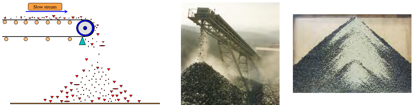
Figure 17.13: a) Sifting and winnowing of coarse and fine material in a conical stockpile (40Pitard, F, 2009.), and b) separation of coarse and fine materials on a stockpile http://www.rohstoffe.rwth-
