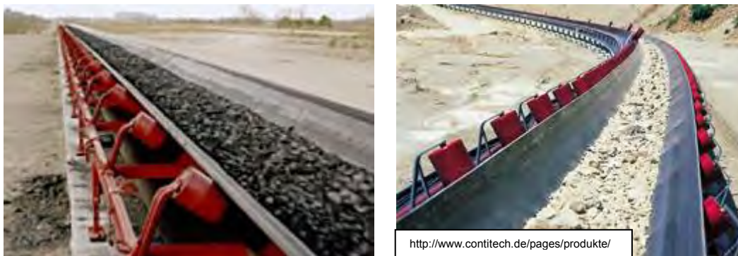
Figure 3.5: Conveyor belts carrying particulate materials reduce the sampling dimensions of the lot to one dimension that can be easily cut by cross-stream or cross-belt samplers.
