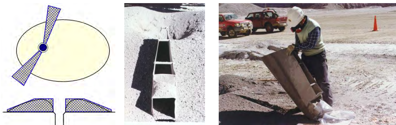
Figure 19.7: a) Use of a radial bucket for RC drill cuttings (40Pitard, F, 2009.) , b) radial bucket in place, and c) being emptied
