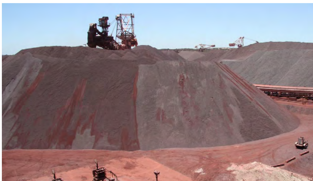
Figure 8.6: Segregated streaks of finer material (light red) across the sides of an iron ore stockpile, Saldanha Bay (used by permission Kumba Resources, 2010).
