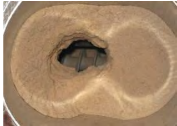
Figure 17.18: a) Prolonged storage and build-up of stagnant material inside a container, b) example of ratholing in a silo. http://www.power-eng.com/articles/print/volume-117/issue-3/features/prb-coal-material-handling-challenges-and-solutions.html
