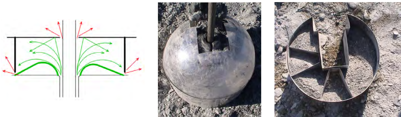
Figure 20.2: a) Example of measures to prevent loss of fines at the mouth of a blast hole(40Pitard, F, 2009.), b) and c) cover design by Ana Carolina Chieregati, Proactive reconciliation in the mining industry , 3rd WCSB, Brazil 2010
