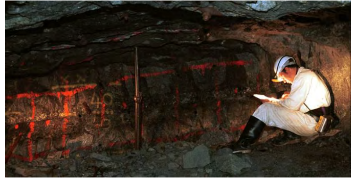
Figure 19.9: a) Sampling should be done at right angles to the mineralised vein and high- grade portions should be avoided when taking waste samples( 40 Pitard, F, 2009.), and b) mapping and sampling a flat dipping reed on South African precious metal deposit
