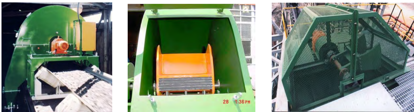
Figure 19.14: a) Cross belt sampler on a conveyor in coal industry b) brush or rubber wiper at the tail-end of the cross-belt cutter and c) a cross-belt cutter or go-belt in a gold plant ( Multotec SA )
