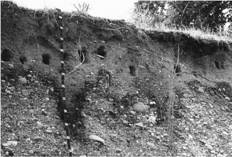
Fig. 12.10 A soil from Michigan with a pronounced concentration of illuvial clay and sesquioxides at a sand-over-gravel lithologic discontinuity. Units on tape are 10 cm. Photo by RJS.
