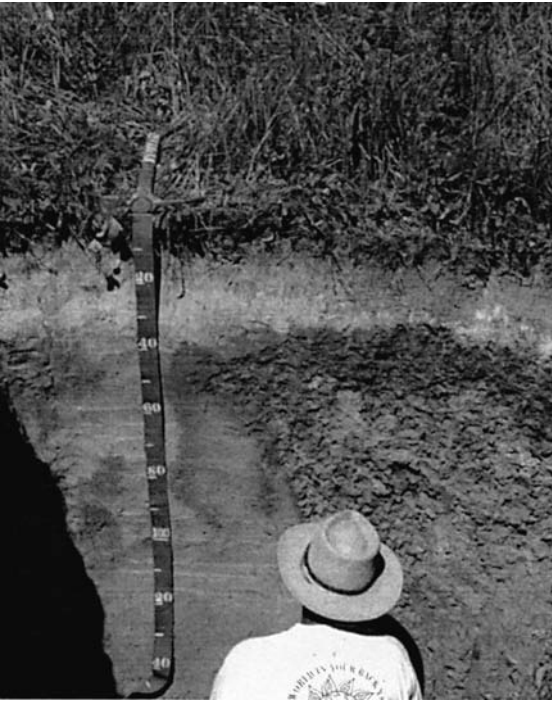
Fig. 7.1 An abrupt soil boundary. The pedon at the left has formed in sandy glaciofluvial sediment, while the one at the right has formed in clayey glaciolacustrine sediment. This abrupt contact formed as meltwater traversing the lake plain ripped gullies into it, and later filled them with sand. Presque Isle County, Michigan. Photo by RJS.
