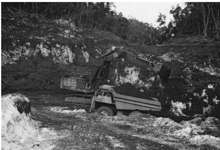
Fig. 8.2 Mining bauxite-rich limestone “residuum” in Jamaica. The ore here is, essentially, the lower profile of an Oxisol. Photo by RJS.
