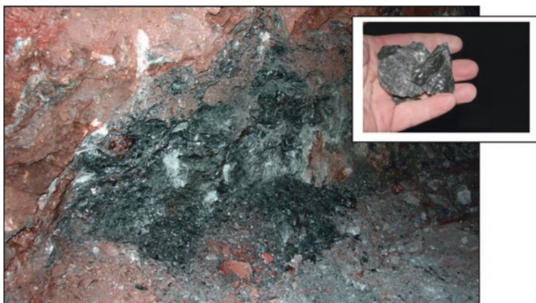
Fig. 19.11 Characteristic view of schistosed serpentinites consisted of slippery laminar pieces and small flakes of millimetres in size (Type IV in Fig. 19.14)
