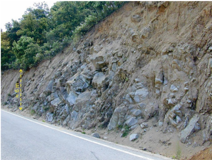
Fig. 11.1 Exposure of physically and chemically weathered granodiorite (an intrusive, igneous rock comparable to granite); zones of fresh, hard, and strong granodiorite (bluish-grey colored) occur in between zones with granodiorite fallen apart in smaller blocks and zones completely decomposed into loose soil material (brownish colored). Note the general increase of decay upwards to the original topographical surface (vegetated) (Road T710, Falset—Gratallops, Catalunya, Spain; photo courtesy of W. Verwaal 2002)
