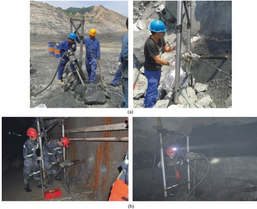
Fig. 7.14 Field application of sampling drill (He et al. 2018). (a) Application at Nanfen open iron mine (Liaoning, 2012). (b) Application at Shajihai coal mine (Sinkiang, 2012)
