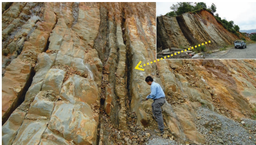
Fig. 11.7 Different lithologies with different susceptibility to weathering result in groundmasses with layers with different states of weathering. The grey, light-brown sandstone is more resistant to weathering than the dark-brown, black shale that is already completely weathered and partially eroded within 5 years after excavation giving the inserts in the groundmass (Flysck deposit of sandstone layers mainly consisting of quartz grains, alternating with shale; Kota Kinabalu, Malaysia, 2011)
