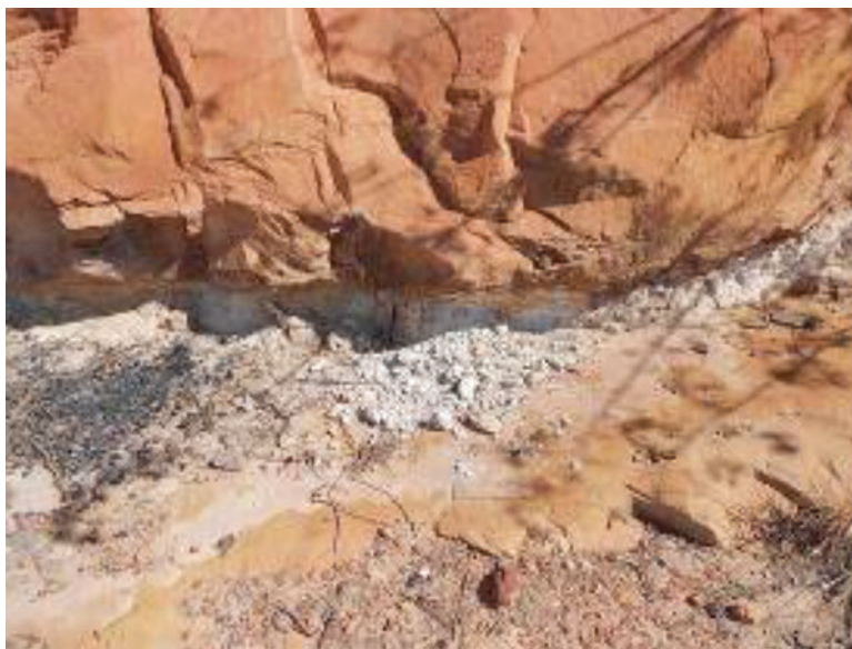
Fig. 5.9 Interbedded weathering silt material in sound sandstone foundation (Photo E.L. Pastore)
