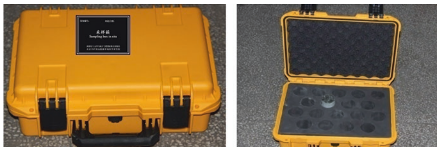
Fig. 7.21 The portable sample box (He et al. 2018)
