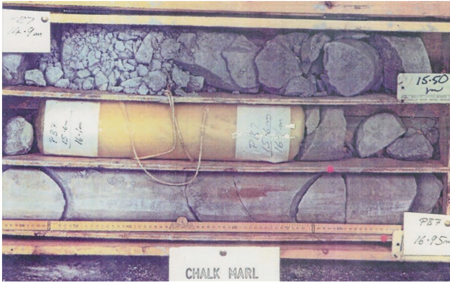
Fig. 18.2 Photograph of PB7 drill core, depth 14.9–16.95 m. Note three joint orientations
