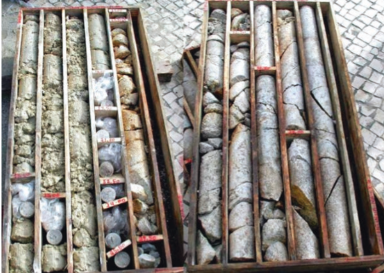
Fig. 7.3 Different borehole samples of Porto granite at Metro do Porto (Babendererde et al. 2006)
