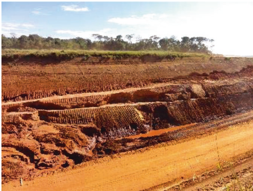
Fig. 5.1 Friable sandstone strata (C4) interspersed into more resistant sandstones with “pits” formed by internal erosion ( piping ). (Photo E.L. Pastore)
