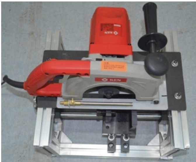
Fig. 7.18 Portable sample cutting machine (He et al. 2018)
