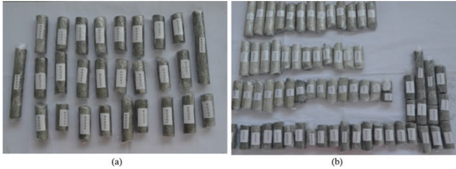
Fig. 7.15 Samples drilled in field (He et al. 2018). (a) Chlorite amphibolite at Nanfen open iron mine. (b) Silt rocks at Shajihai coal mine
