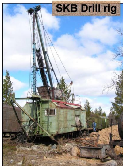
Fig.5. License area is poorly outcropped. Auxiliary methods and geological mapping were not very informative under these conditions, and the main information about PGE mineralization was received with drilling. More than 200 diamond drill holes (DDH) were drilled in the area, average depth of DDH was 150 meters, the deepest – more than 500 m.
