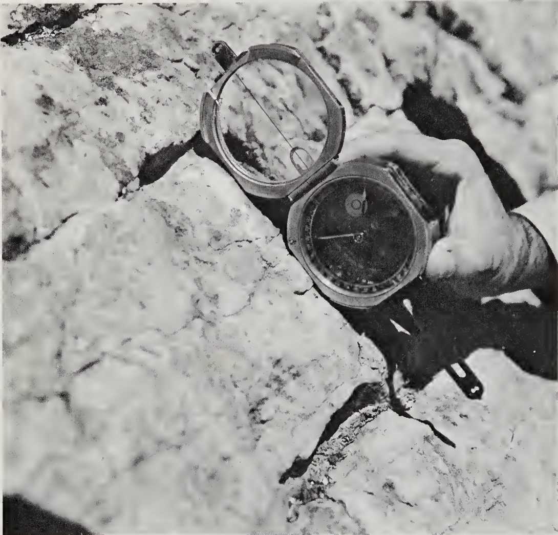
Plate 2. Measuring dip. Dakota Sandstone. Usually the geologist stands at a distance to eliminate effect of small irregularities in the bedding. Colfax County, New Mexico. Photo : J. R. Stacy, U. S. Geological Survey.
