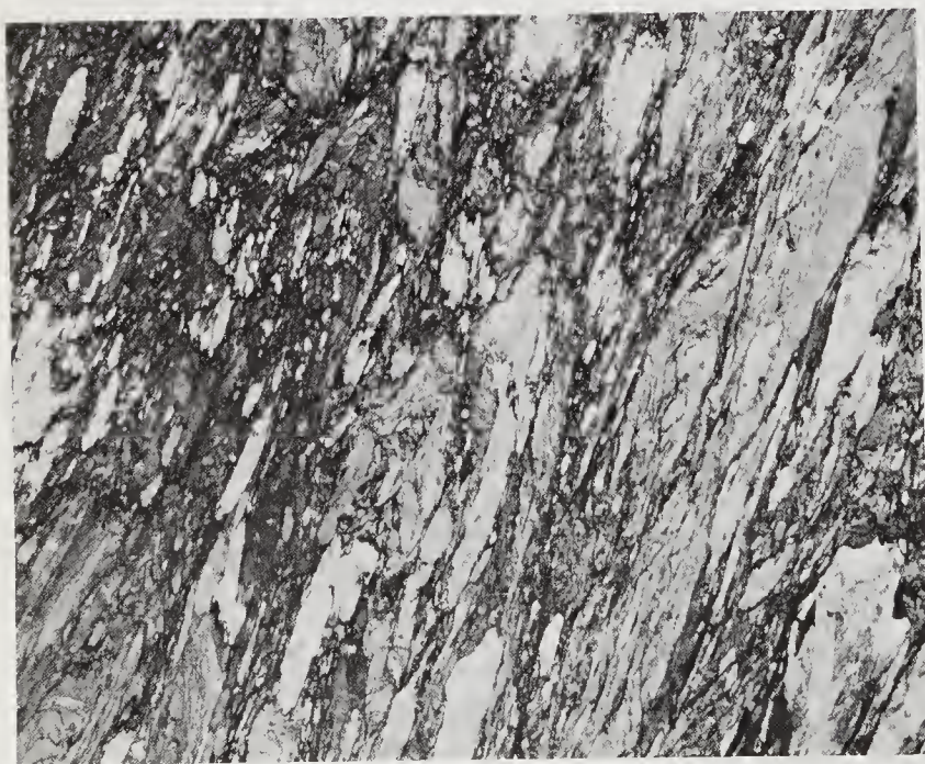
Plate 20 Photomicrograph of tectonic breccia. About 2 centimeters across. Derived from slate and chert along Melones fault zone. Dutch Flat Quadrangle, California. Photo: L. D. Clark, U. S. Geological Survey.
