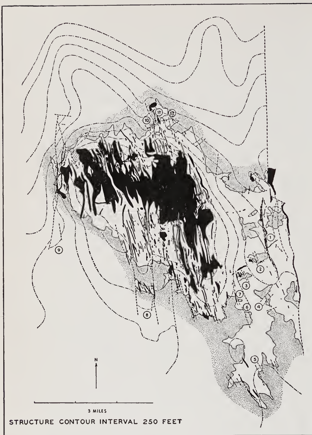
Fig. 17-6. Doming by forceful intrusion. Black Hills of South Dakota. Black represents rhyolite of Tertiary age. Stippled area is the base of the Paleozoic strata (only the base of the Paleozoic is stippled; the white area outside the stippled area is Paleozoic and Mesozoic). White inside of the stippled area represents Precambrian. Dash-dot lines are structure contours on base of Paleozoic; contour interval 250 feet; greatest uplift is in center of area. Numbers in circles refer to small horsts uplifted between paired faults (short dashes). (After J. A. Noble; permission of University of Chicago Press.)
