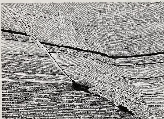
Fig. 11-16. Edge of an artificial graben. Produced by subjecting clay to tension. The master fault and many subsidiary faults dip to the right. Antithetic faults dip to the left. All the faults are of the gravity type. (After H. Cloos. 12 )
