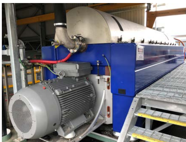
Figure 6: 1,000 mm solid bowl centrifuge supplied by Alfa Laval
