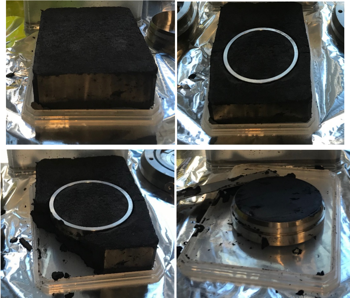
Figure 3: Coal tailings specimens being cut for oedometer testing
