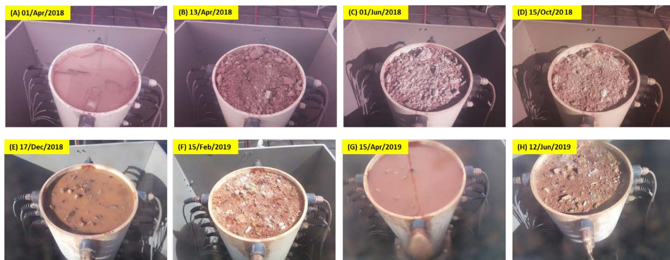
Figure 5: Images of column surface at different stages of the test
