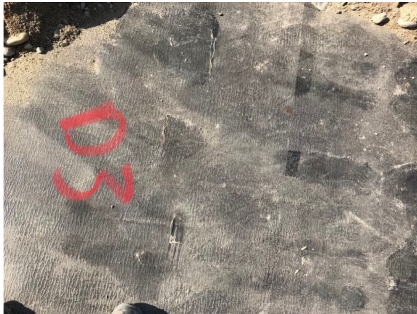
Figure 7: The BGM surface after compaction with D3 dozer over 0.4 m of fill with cobbles
