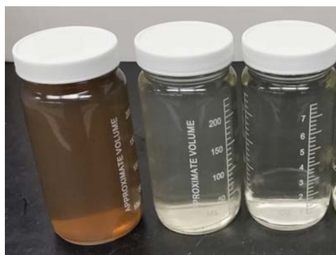
Figure 6: Release water from GC1 (HPAM, left) and GC2 (XUR, middle and right)
