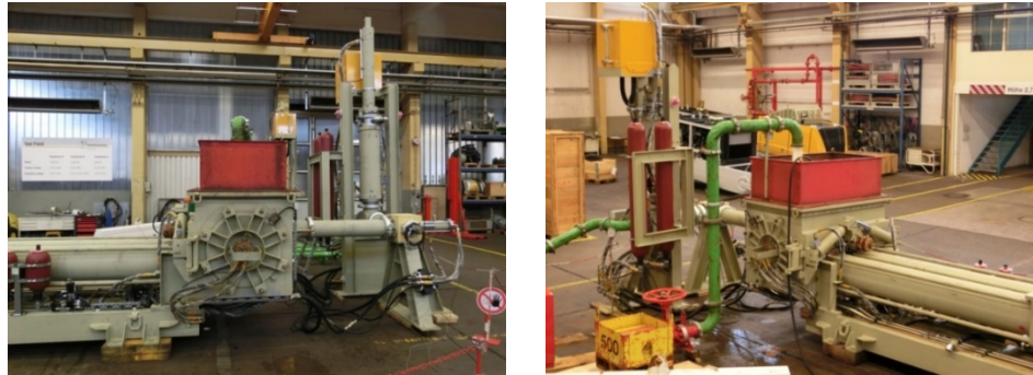
Figure 8: Hydraulic driven S-tube pump with an hydraulic pulsation dampening system
