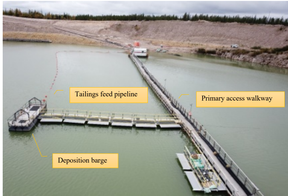
Figure 4: Subaqueous field trial configuration
