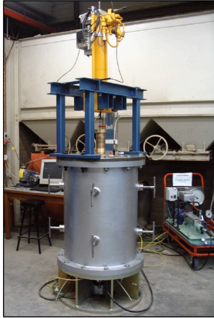
Figure 2: View of the calibration chamber at UNSW (the chamber itself has an outer diameter of approximately 0.7m)
