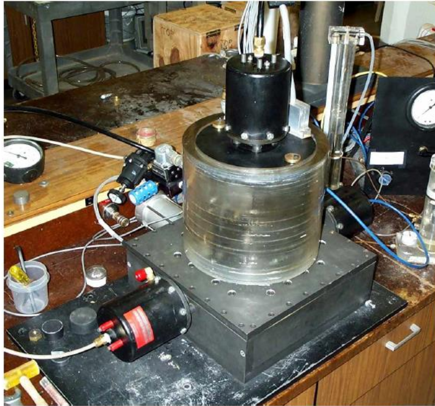
Figure 2: Bidirectional cyclic simple shear device (Kammerer et al., 2004)
