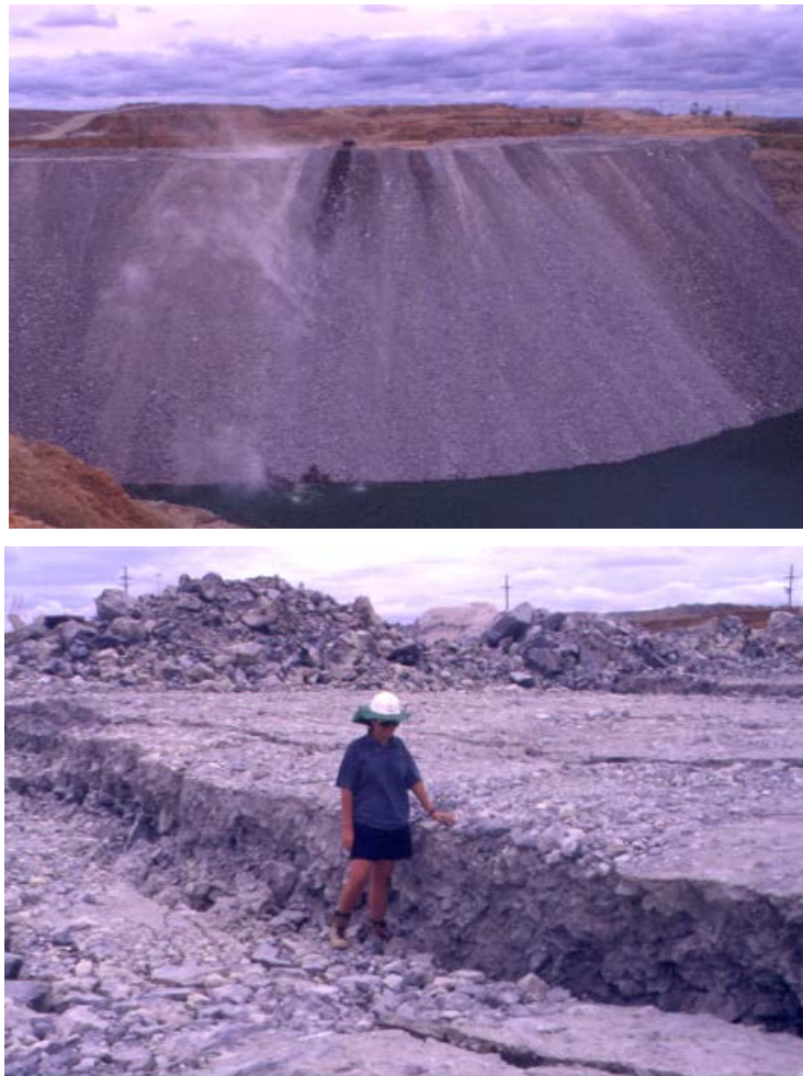
Figure 9: End-dumping waste rock in-pit at Kidston Gold Mines: (above) 240 m high dump face, and (below) scarps up to 1 m high formed at crest reflected from pit slope benches
