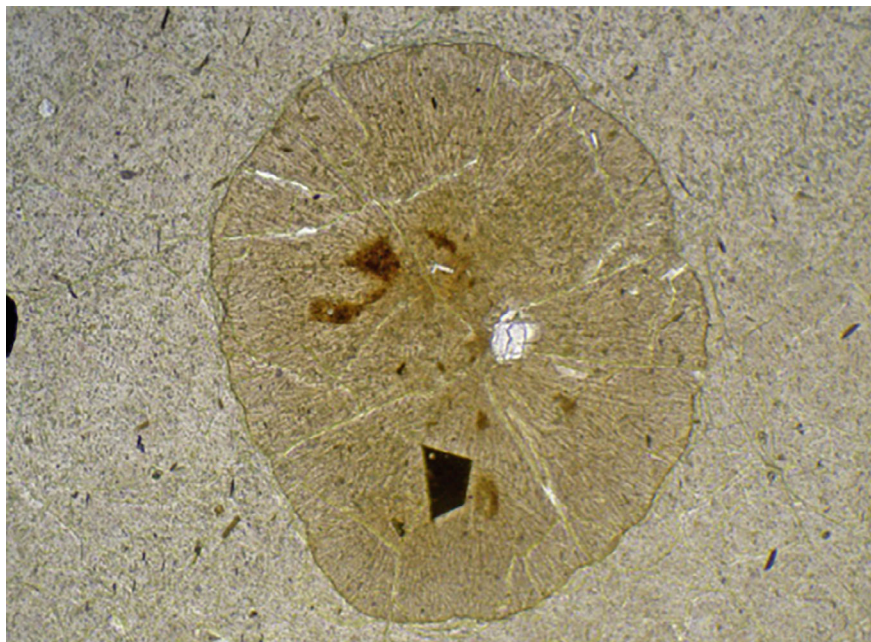
Fig. 3.6 Devitrification spherulite in volcanic glass showing radial structure; plane light (ufgrs. br, Feb. 2022)
