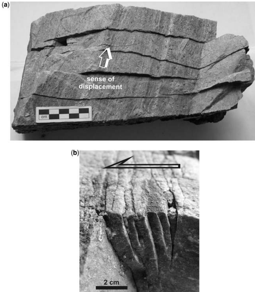
Fig. 6. (a) View onto the foliation plane forming the shear zone boundary of a chlorite-bearing quartzite from the Palten–Liesing fault. The step traces on the foliation plane are formed by fractures at high angle to the fault zone boundary. (b) View perpendicular to the shear zone boundary, showing slightly bent lamellae confined by subvertical fractures. Both samples are from the site 'Mautern' (see Appendix 1).
