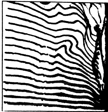
Fig. 14.4. Bubble isochrones (that is, lines of constant time; side view) in boundary layer around flat plate. Bubbles generated by vertical wire (left edge of photo, flow from left to right).
