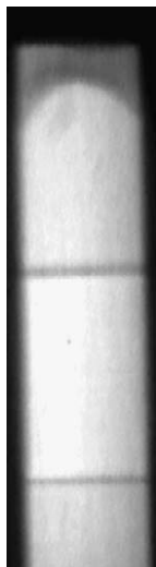
Figure 5 Shadowgraph image of a sample at high pressure and temperature. The black boundary is defined by tungsten carbide anvils; the dark lines are from metal foils within the sample.
