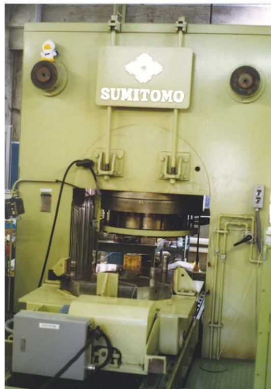
Figure 9 Photos of Kawai-type pressure apparatus installed at ISEI, Okayama University. (a) Lower half part of the guide block make up of three bound split spheres. The Kawai cell covered by mica sheets is set at the center. (b) A 5000 ton press to drive the split sphere guide blocks.
