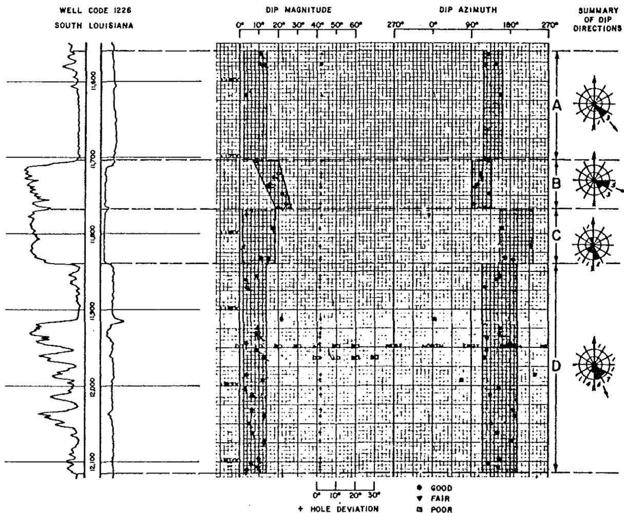
The massive sand below 11,700 feet on the log appears to be a single thick sand unit on casual inspection of the E-log. The dipmeter log, however, shows a distinct change in the dip pattern between Units "B" and "C". This change in dip pattern is evidence that Sand Units "B" and "C" are two separate and distinct sand bodies. A re-evaluation of the E-log shows slight differences in log character between the upper and lower parts of the sand.
