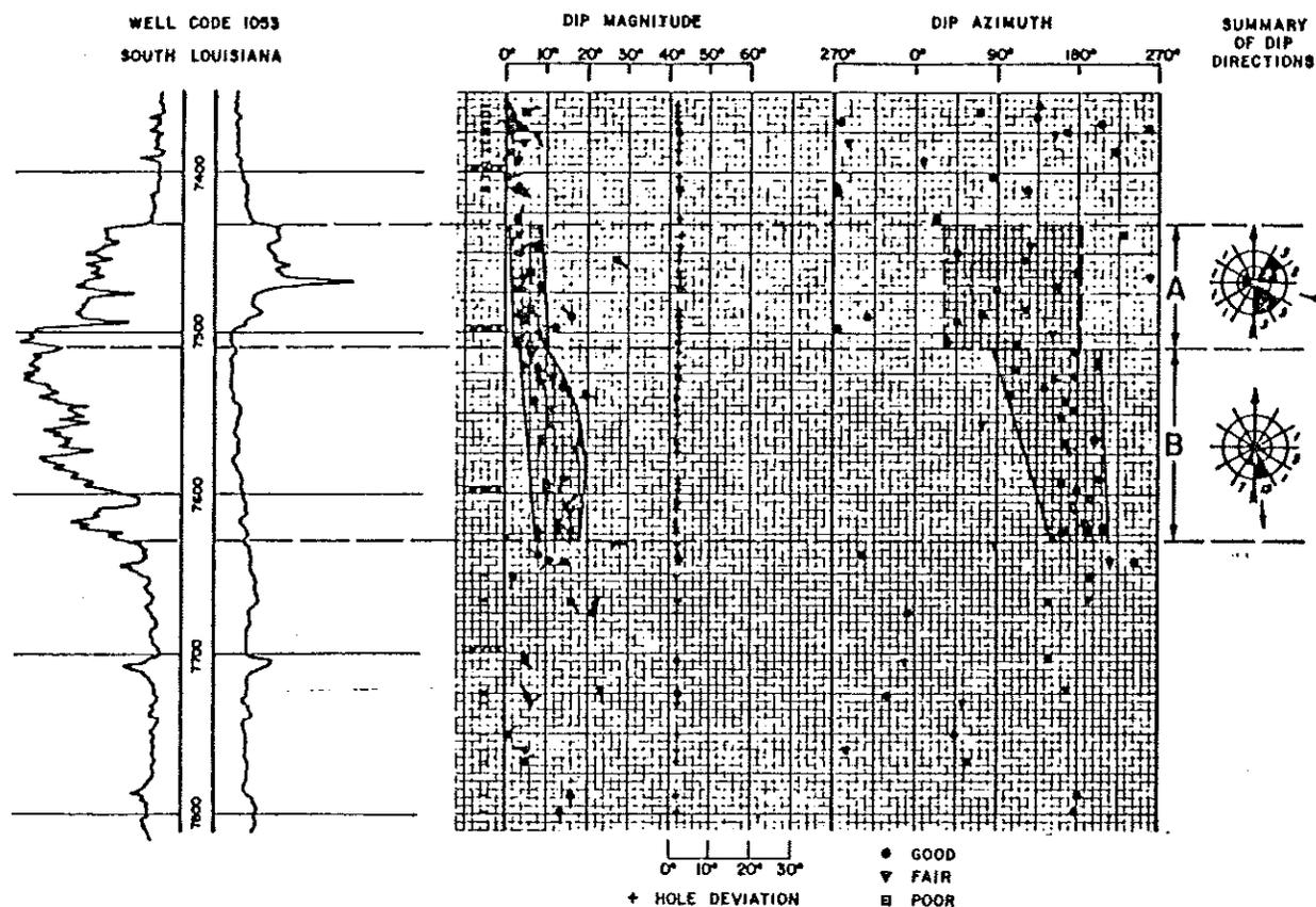
The dips in Sand Unit "B" range in magnitude from about 4° to 20° and form a prominent southerly directional pattern. In contrast, the dips in Sand Unit "A" are generally lower (except for 3), and they form a less consistent directional trend. The structural dip of about 2° southeast at this location was determined from subsurface mapping.
