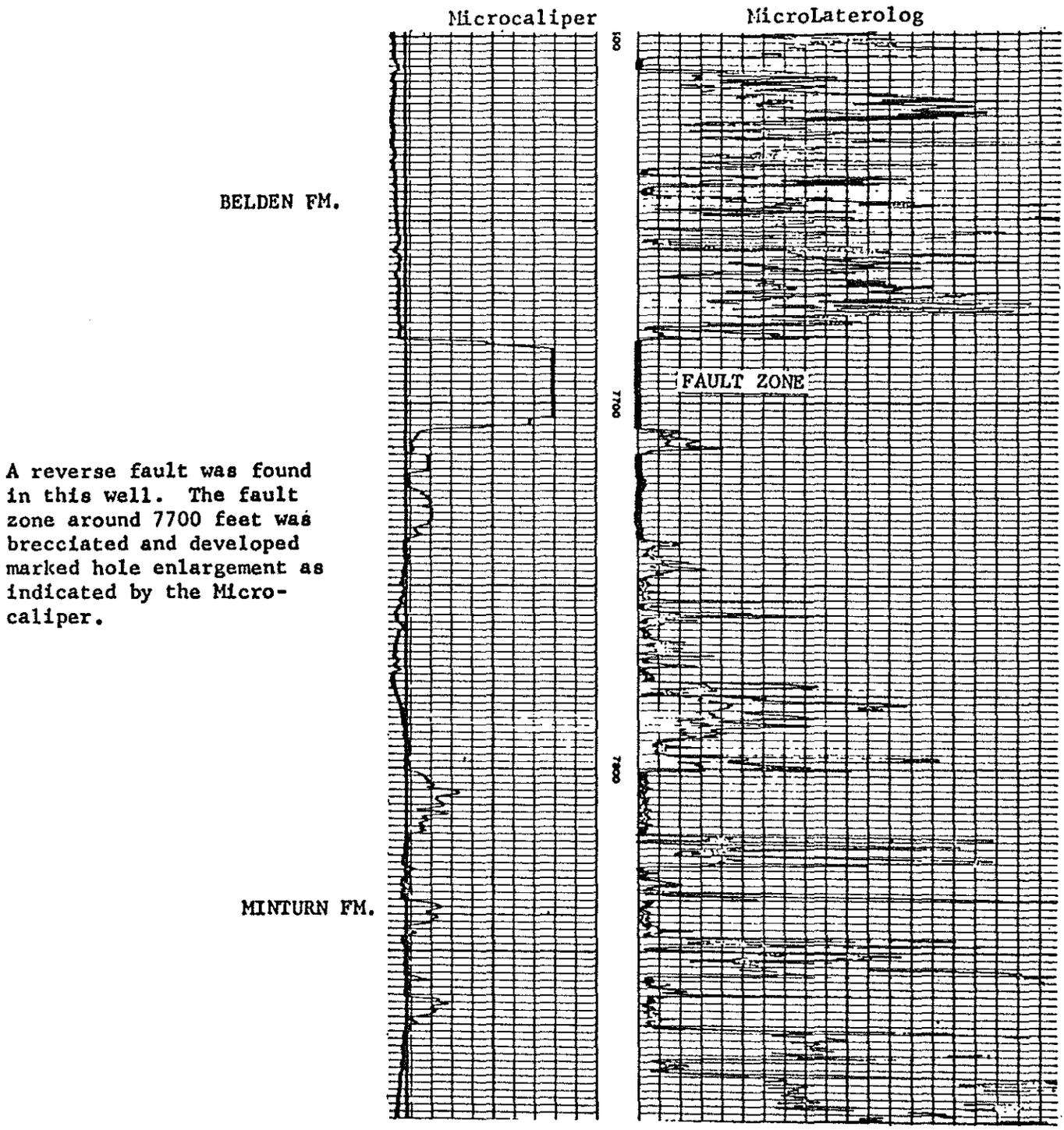
A reverse fault was found in this well. The fault zone around 7700 feet was brecciated and developed marked hole enlargement as indicated by the Microcaliper.
