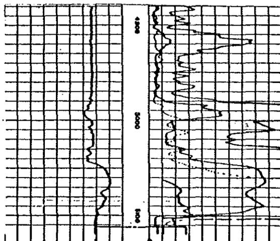
Reversed SP resulting from the formation water being fresher than the mud filtrate.
