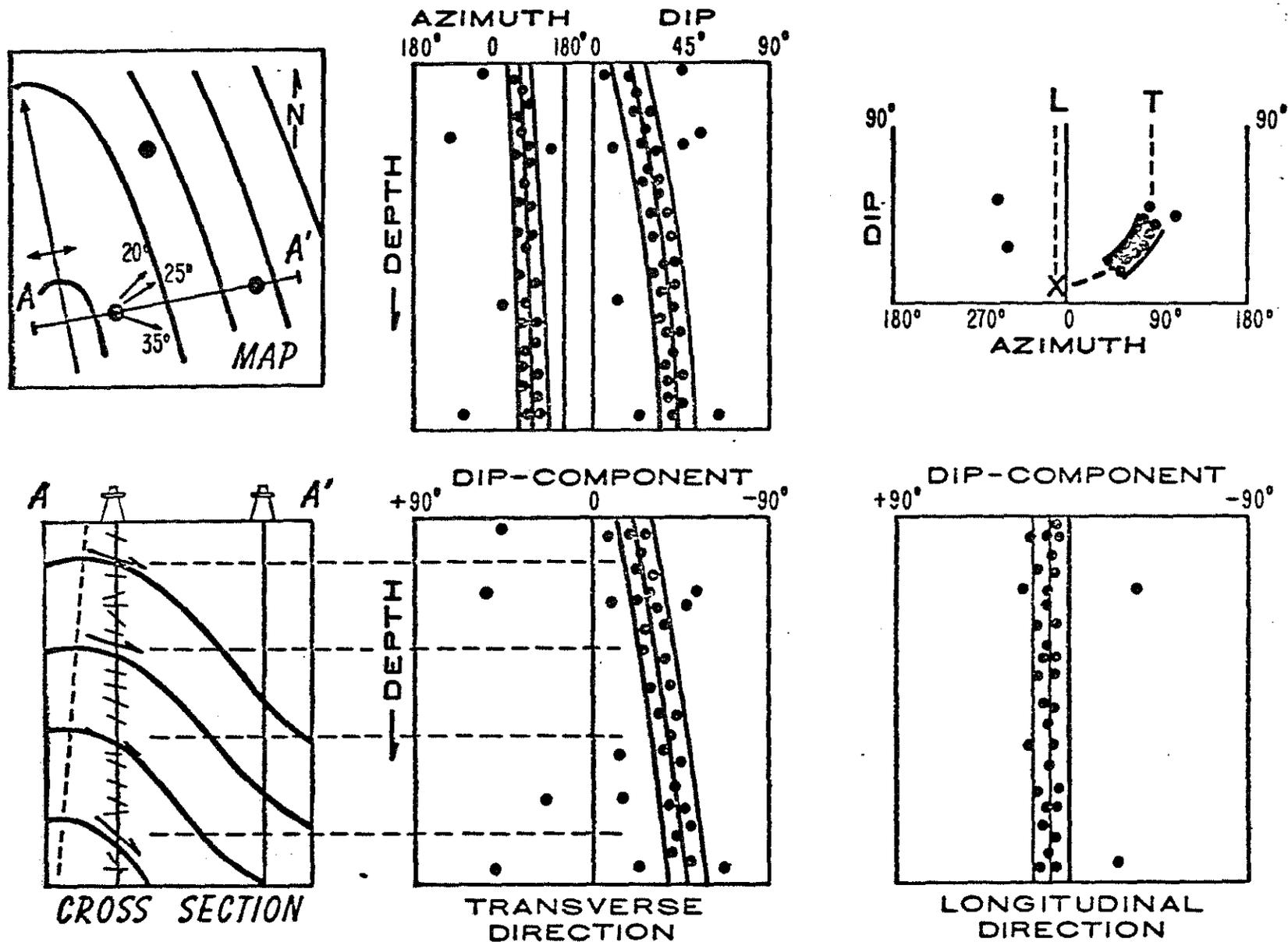
VECTOR AND GRAPH-TYPE DISPLAYS OF DIPMETER DATA
