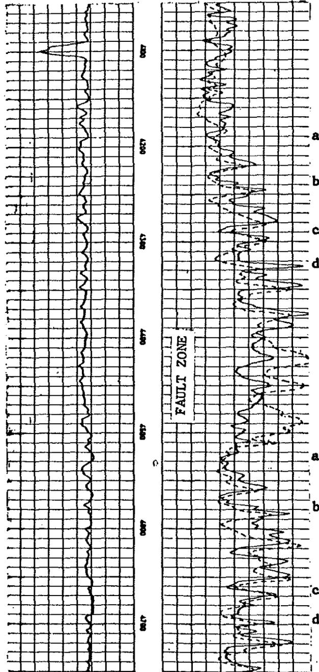
Note use of short normal for correlation. Correlations a, b, c, and d show bed repetition from reverse faulting. Correlation is based entirely on electrical resistivity character.
