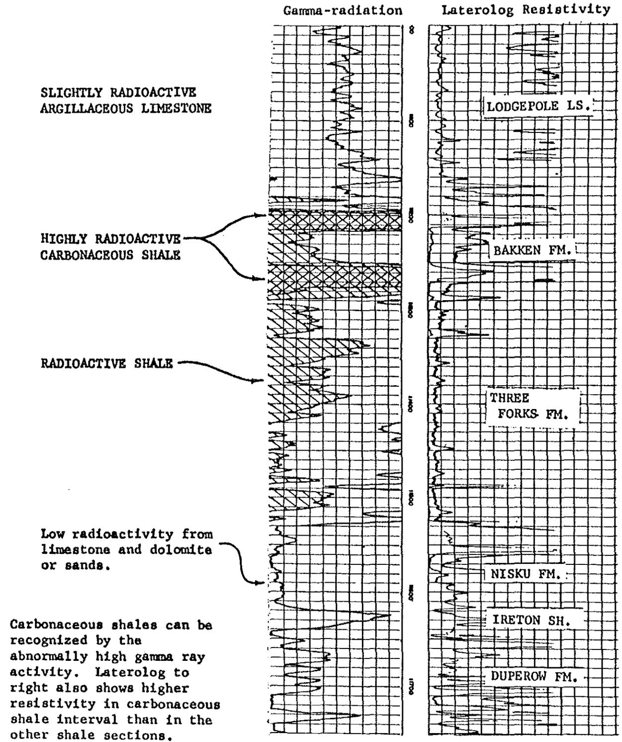
Carbonaceous shales can be recognized by the abnormally high gamma ray activity. Laterolog to right also shows higher resistivity in carbonaceous shale interval than in the other shale sections.
