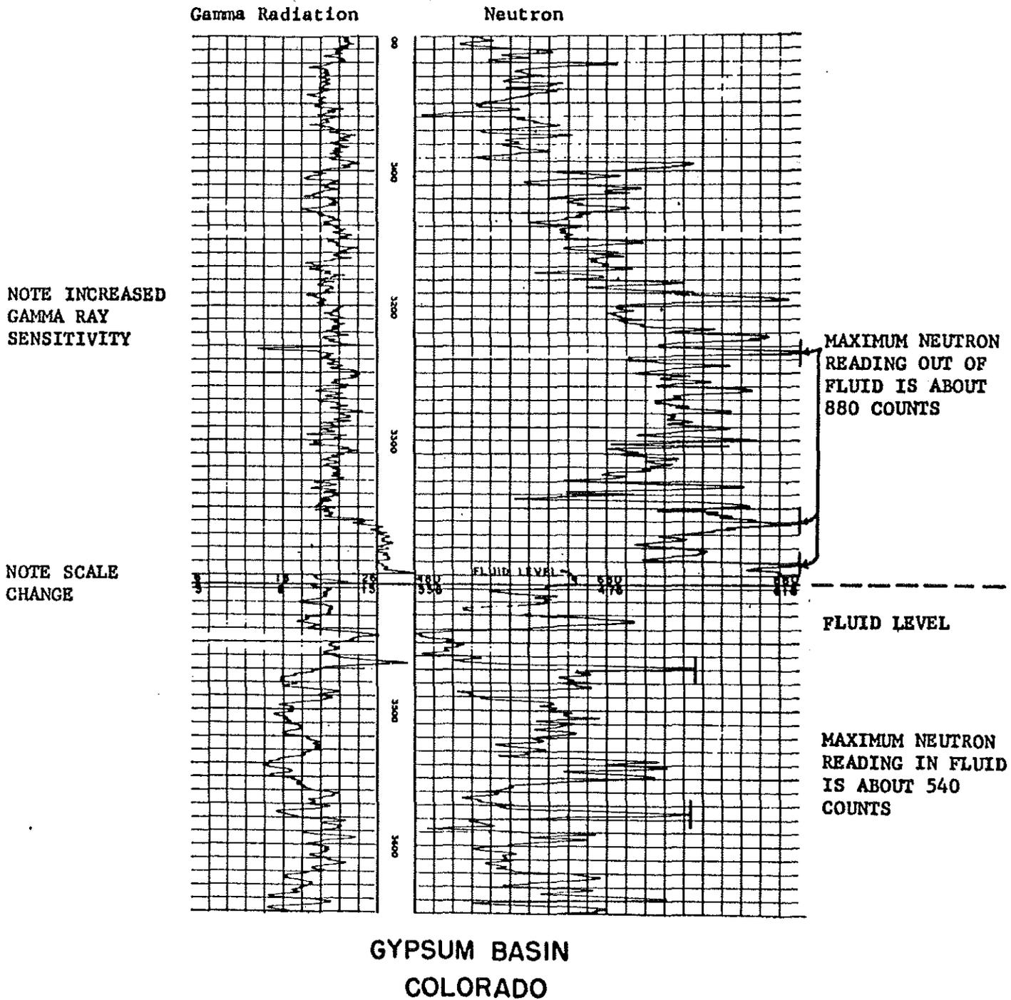
Well bore fluid depresses gamma ray and neutron activity. Unmarked fluid levels may resemble formational boundaries.
