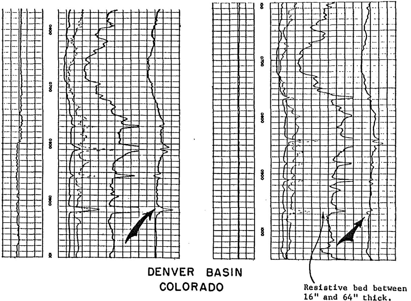
Interval 910-920 feet on log to left shows a resistive bed on all three curves. Log on right side shows a well defined resistive bed only on the lateral curve. The long normal on the right hand log is affected by critical bed thickness and actually shows resistivity reversal. Normal curves always show resistivity reversal in beds of high resistivity when the bed thickness is less than the log spacing. When correlating by normal curve character, the bed thickness should be considered.
