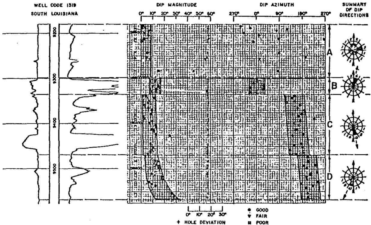
The dips in Units "A" through "D" on Figure 2-21 have been replotted after removal of the effects of structural tilting. The structural dip in Unit "A" was assumed to be 3° S 15° W. The dip in Units "B", "C" and "D" was assumed to be 7° south.
