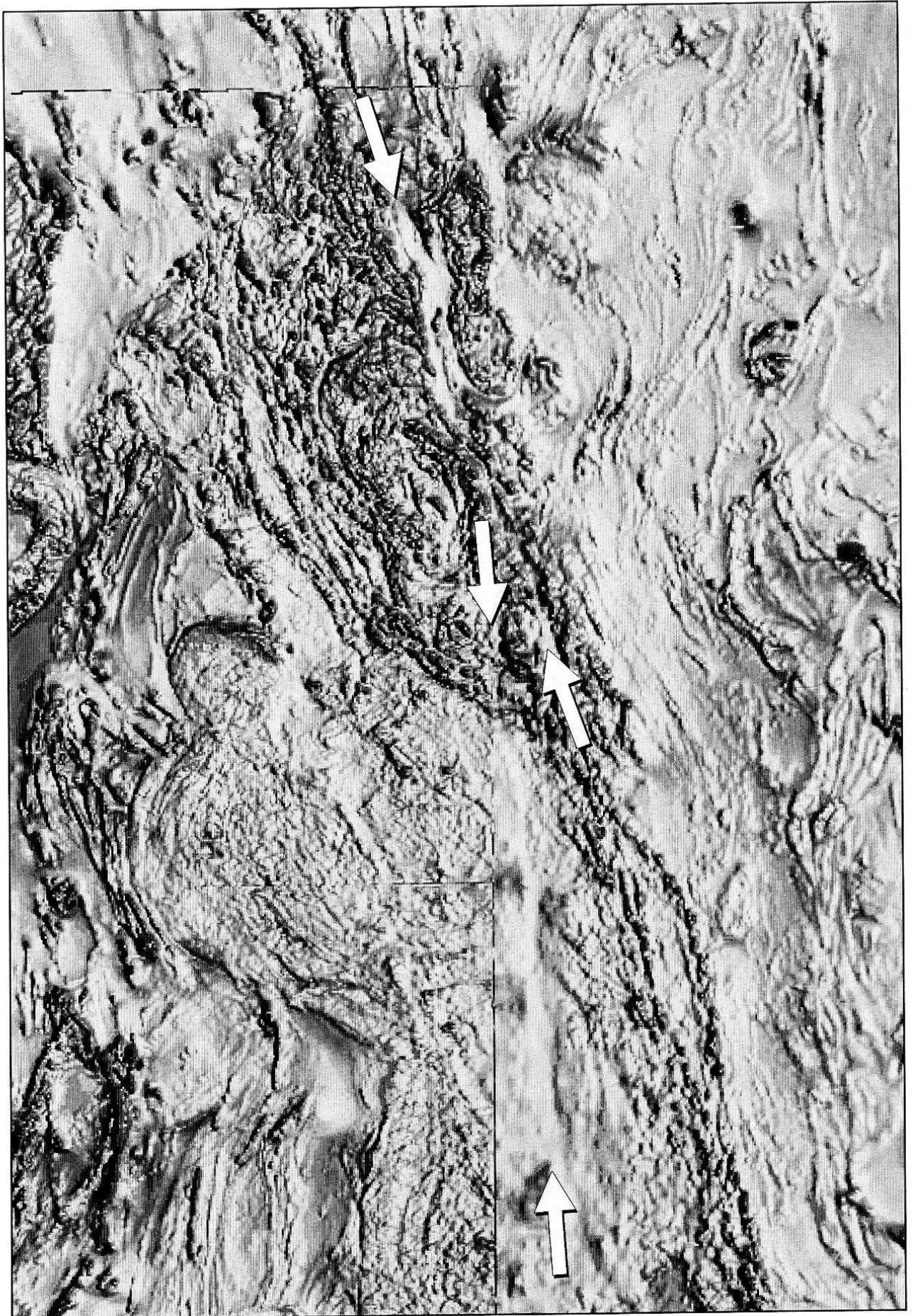
Figure 4: Image of the aeromagnetic data (total magnetic intensity) of part of Eastern Fold Belt, Mt Isa Inlier. The Cloncurry Fault, a major strike fault traverses the area shown, and is evident as a discrete NNW-trending "magnetic valley" extending from the northern to southern limits of the image. The magnetic "valleys" are highlighted with the arrows. The image shows an area approximately 80 km wide
