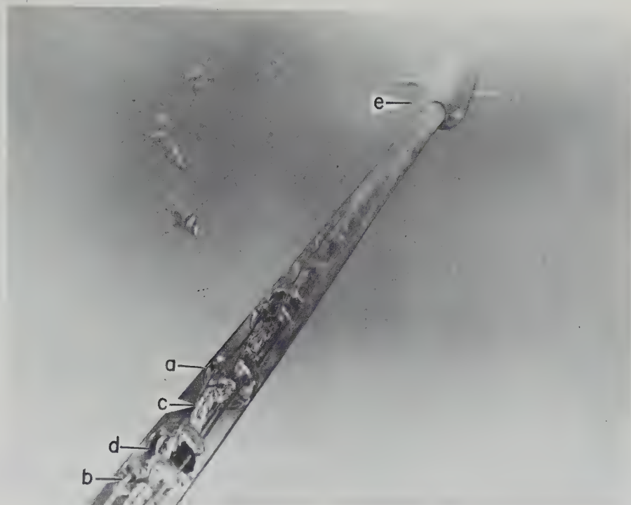
Figure 4.65. Photo of seismic streamer. Plastic spacers (a) are connected by three tensile cables (b). A bundle of electrical conductors (c) passes through holes in the centers of the spacers. A hydrophone is at (d). A depth controller (e) is clamped over the streamer (Courtesy Seismic Engineering.)
