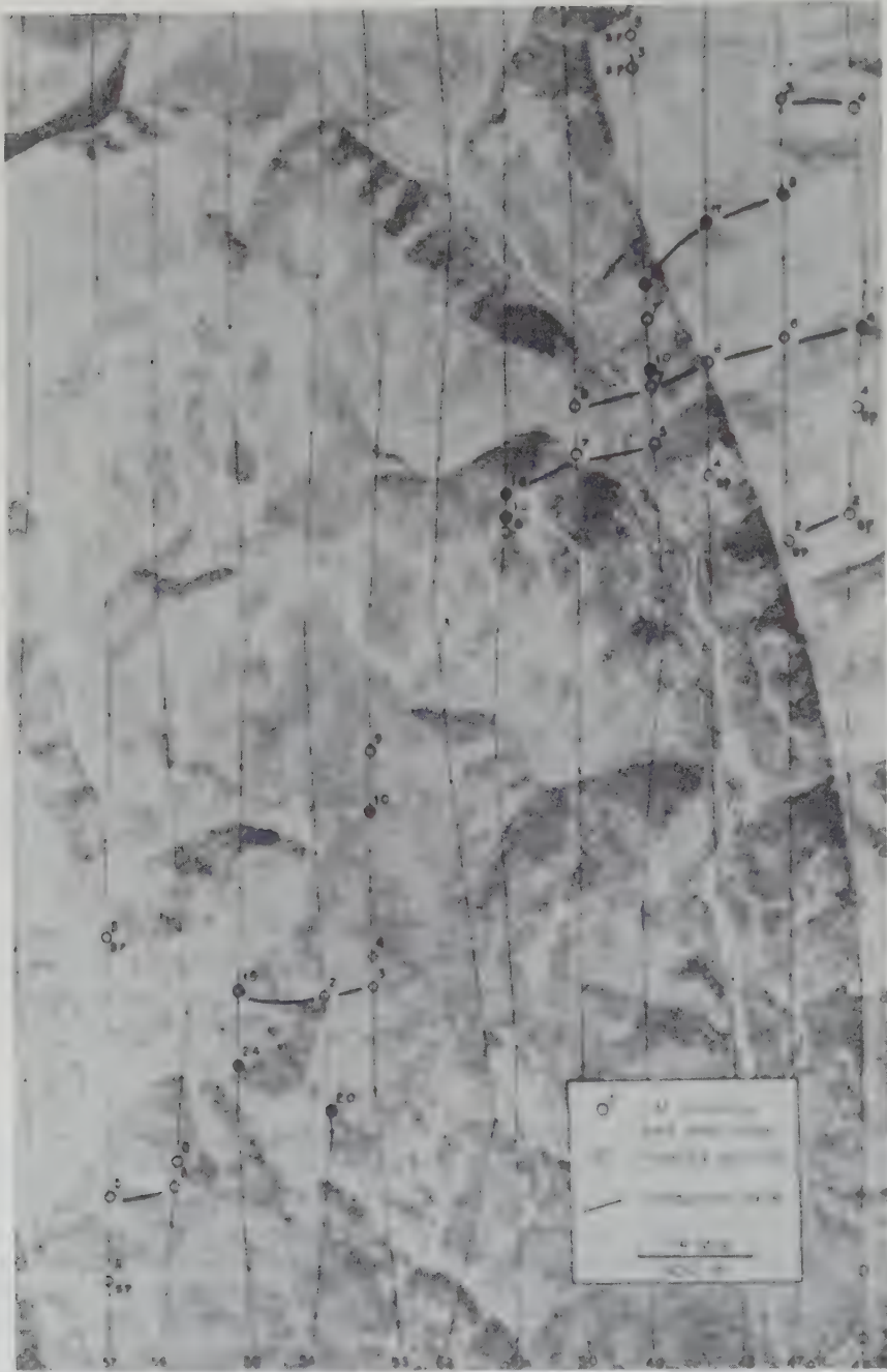
Figure 7.123. Airborne EM (Dighem II) map of an area in the Appalachians.
