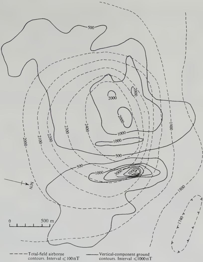
Figure 3.41. Comparison of ground vertical-component data with airborne total-field data.
