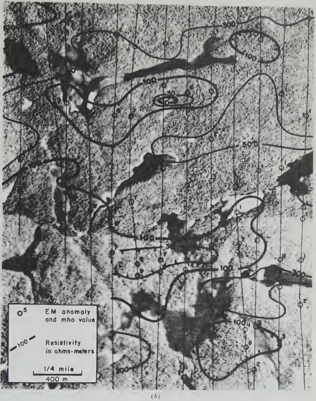
Figure 7.85. (Continued) (b) Pseudolayer resistivity map of the area in (a) showing two bedrock conductors.
