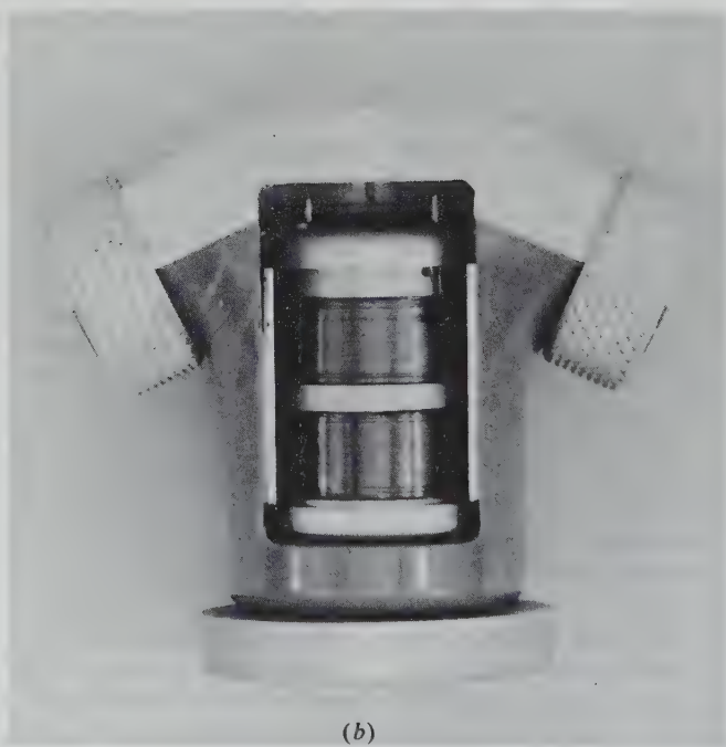
Figure 4.53. Moving-coil geophone. (a) Schematic. (b) Cutaway of a digital-grade geophone. (Courtesy Geo Space Corp.)
