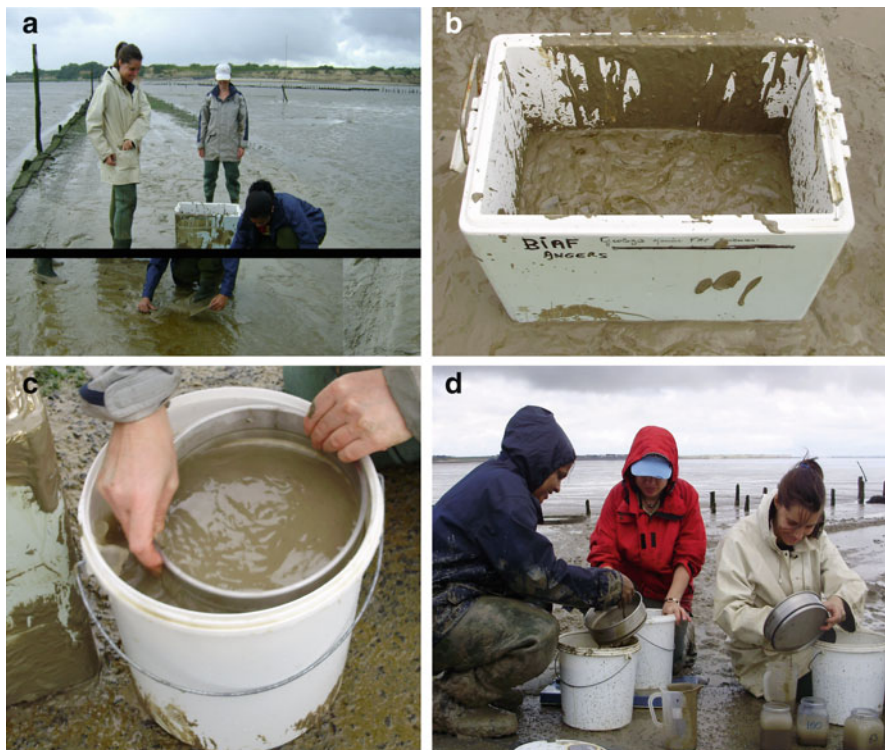
Fig. 8.1 Various steps in the initial treatment of sediment samples in the field: (a) Sediment samples being scooped in to sampling box. (b) Closer look of the collected sample. (c) Preliminary sieving of the samples in the field. (d) Sieved sampled getting transferred to bottles along with seawater
