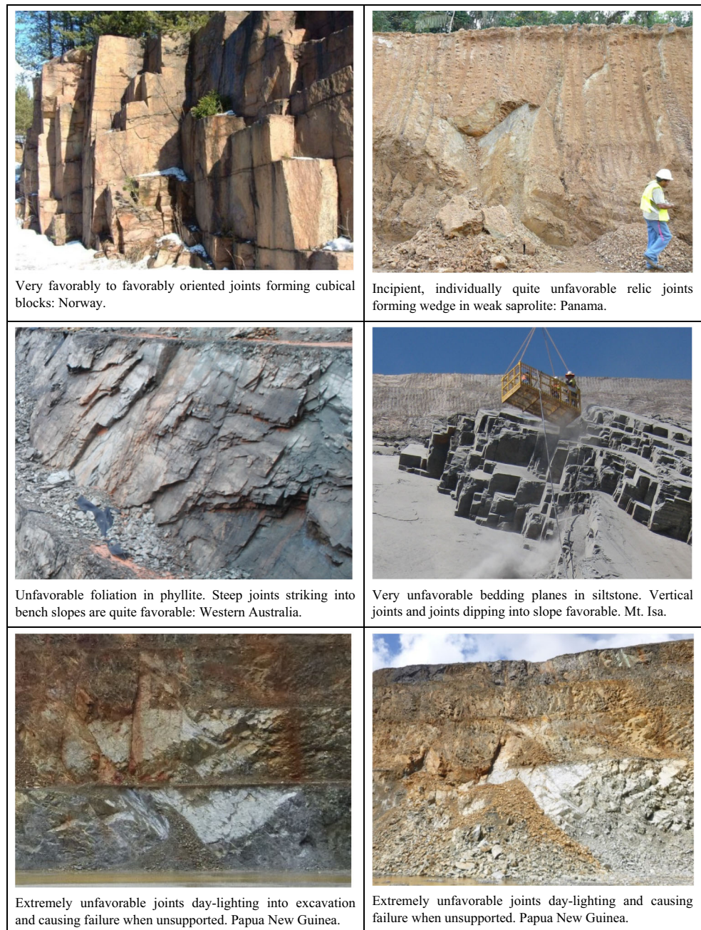
Fig. 7 Examples of the need for O-factor (discontinuity orientation factor) application
