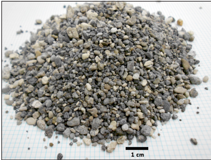
Figure 2.2 Florida sedimentary phosphate ore sample
