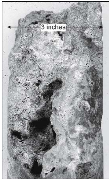
Fig. 1.5. Core sample of a large vug from a Silurian reef, Michigan. The measured permeability from a core plug taken from this sample is <0.1 md, which is an obvious understatement of the permeability of this sample
