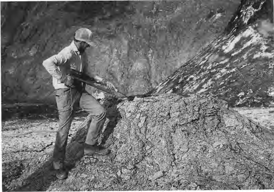
Fig. 2. Hornito 5 filled with frothy lava. The rheological properties of the lava are being measured using the rotating vane viscometer described in the text
