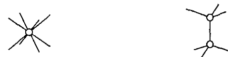
Fig. A3.2. Left: a repeat unit of bcc. Right: the repeat unit of the diamond structure; each bond (except the one in the center) traverses a face of the primitive unit cell.
