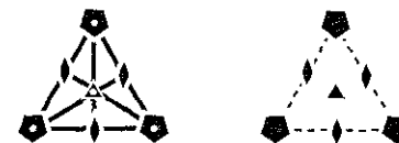
Fig. A4.9. Some of the icosahedral symmetry elements. On the left 2, \bar{3} and \bar{3} axes of I_h are shown with heavy lines representing the traces of mirror planes. On the right are shown the corresponding 2, 3 and 5 axes of I .
