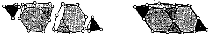
Fig. 6.56. Two tetrahedra and two truncated tetrahedra combining to make a 60^\circ rhombohedron (right).
