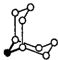
Fig. 7.4. Illustrating two 6-rings containing the same angle (heavy lines) at a vertex (filled circle) in the diamond net. This figure is a fragment of Fig. 7.10 (left).
