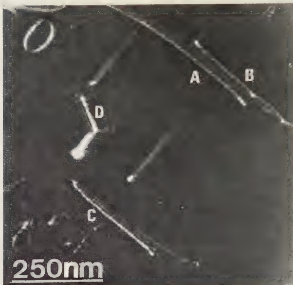
Figure 16.13 Dissociation of dislocations with \mathbf{b} = 1/2[\bar{1}\bar{1}1] (A, B, C, D) in (11\bar{2}) planes into three collinear partials. A, B, and C are screws. A and B form a dipole. D joins a node. Dissociation of screw dislocations with \mathbf{b} = [1\bar{1}0] ( N55^\circ E ) into two collinear partials. In the upper left there is a small loop in the (001) plane with \mathbf{b} parallel to [02\bar{1}] . 3.8 per cent strain at 400^\circ C . CA \approx FN \approx [100] . DF/WB, \mathbf{g} = [0\bar{2}4]^* , BM \approx [221] .
