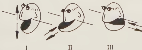
Figure 2.1 The three modes of fracture: I, opening mode; II, sliding mode; III tearing mode.
