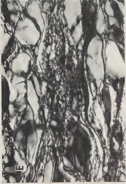
Figure 8.7 Optical photomicrographs of Enfield apfite; all micrographs are the same scale. (A) Starting material: grains with cross-hatch pattern are microcline, grey grains are mostly oligoclase, white grains are mostly quartz, but tabular grain is biotite. (B–D) Samples deformed at 1500 MPa and 10^{-6} \text{ s}^{-1} , with increasing temperature: compression direction is vertical. (B) 47 per cent shortening at 725 °C: dispersed quartz grains (white) remain little deformed, while feldspars have deformed by cataclastic flow. (C) 55 per cent shortening at 800 °C: quartz and feldspars have deformed about equally, the former by climb-accommodated dislocation creep, and the latter by a combination of cataclastic flow and recrystallization-accommodated dislocation creep. (D) 55 per cent shortening at 900 °C: both quartz and feldspars have deformed by dislocation creep, but the latter are stronger and are becoming less connected, while the former is weaker and is becoming interconnected. (E) 85 per cent shortening, 900 °C: portions of relatively undeformed feldspar grains are dispersed, quartz and recrystallized feldspars form interconnected matrix.
