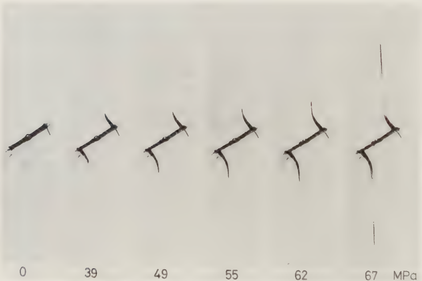
Figure 4.2 A sequence of photographs of wing-crack initiation and growth under progressively higher compressive stress. (Reprinted with permission from Acta Metallurgica 34, Hallam & Ashby, Copyright 1986, Pergamon Journals Ltd.)
