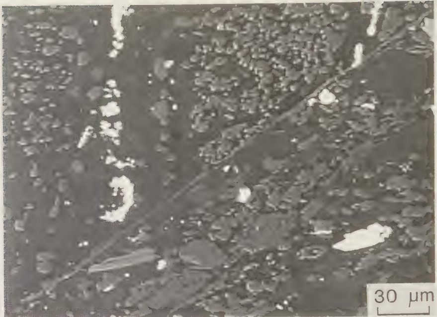
Figure 10.5 Backscattered electron image of serpentine deformed at 500 C (Rutter & Brodie 1988). The dark grey background is serpentine which contains grains of olivine and orthopyroxene (both medium grey), which were present prior to the experiments, as well as newly formed olivine grains up to 10 \mu\text{m} diameter. Two narrow planar shear zones ( \sim 5 \mu\text{m} wide) can be seen which contain fine-grained (0.1–0.2 \mu\text{m} diameter) olivine. Most of the deformation occurred in such shear zones. The very bright grains are Fe oxides.
