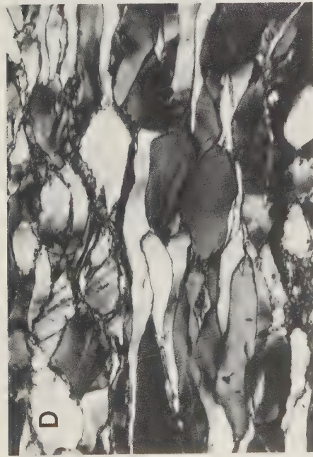
Figure 8.7 Optical photomicrographs of Enfield apfite; all micrographs are the same scale. (A) Starting material: grains with cross-hatch pattern are microcline, grey grains are mostly oligoclase, white grains are mostly quartz, but tabular grain is biotite. (B–D) Samples deformed at 1500 MPa and 10^{-6} \text{ s}^{-1} , with increasing temperature: compression direction is vertical. (B) 47 per cent shortening at 725 °C: dispersed quartz grains (white) remain little deformed, while feldspars have deformed by cataclastic flow. (C) 55 per cent shortening at 800 °C: quartz and feldspars have deformed about equally, the former by climb-accommodated dislocation creep, and the latter by a combination of cataclastic flow and recrystallization-accommodated dislocation creep. (D) 55 per cent shortening at 900 °C: both quartz and feldspars have deformed by dislocation creep, but the latter are stronger and are becoming less connected, while the former is weaker and is becoming interconnected. (E) 85 per cent shortening, 900 °C: portions of relatively undeformed feldspar grains are dispersed, quartz and recrystallized feldspars form interconnected matrix.
