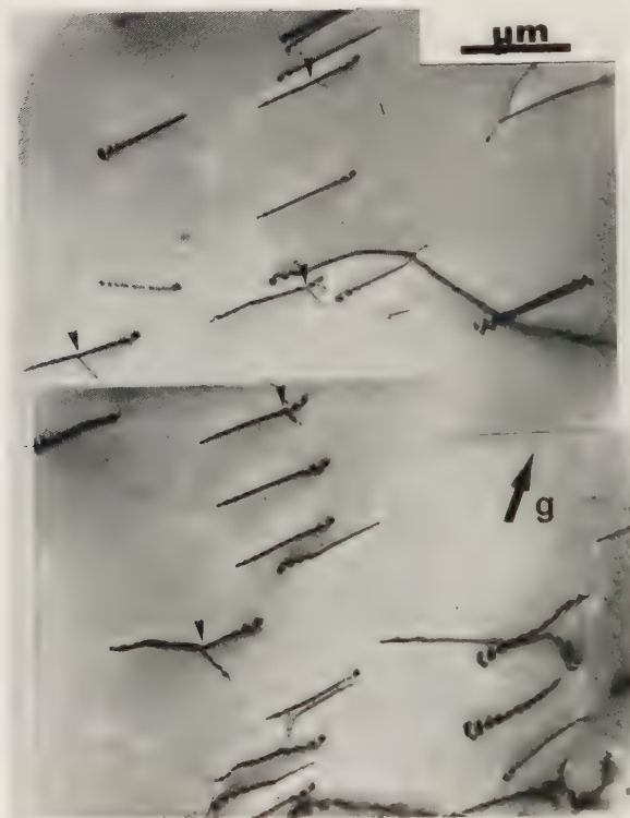
Figure 16.7 Dislocations parallel to [110] in the (\bar{1}12) and (001) planes. At triple junctions ( \leftarrow ) several dislocations are joined by [110] directed segments. Most of these junctions result from dipole interactions of dislocations with \mathbf{b} = [\bar{1}\bar{1}0] . 1 per cent strain at 200^\circ\text{C} . \text{CA} \approx \text{FN} \approx \text{BM} \approx [021] , \text{BF} , \mathbf{g} = [024]^* .
