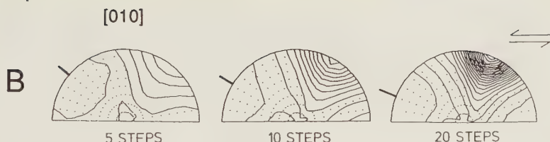
Figure 14.3 [010] axis diagrams for simple shear, model B, illustrating the effect of increasing shear. Each step corresponds to an incremental shear of 0.1. The direction of the longest finite strain axis is indicated. Contour interval 0.25 m.r.d., dotted below 1 m.r.d.
