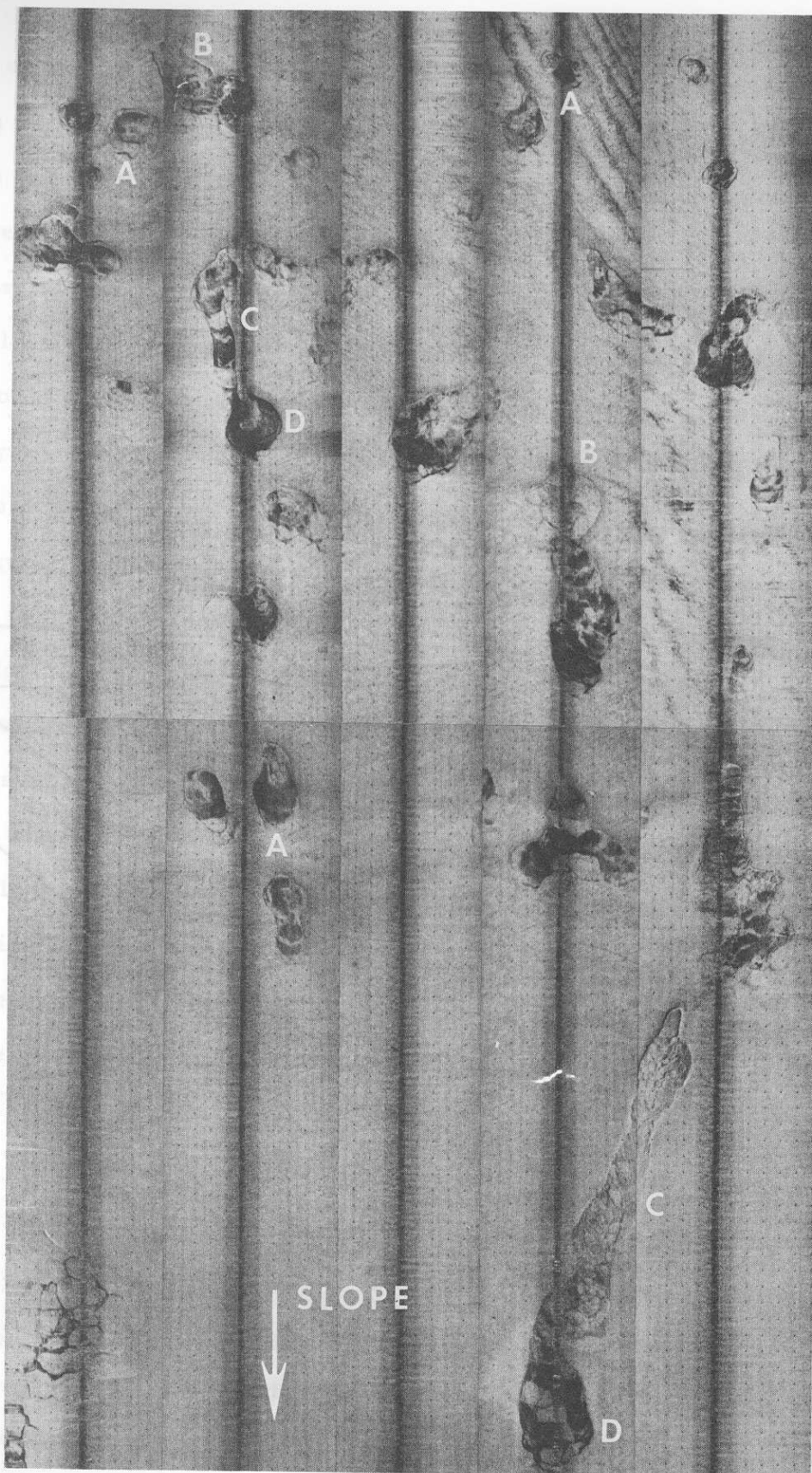
Figure 38. Side-scan sonar mosaic illustrating several collapse depressions and a bottleneck slide. The grids are 25 m apart and the mosaic covers an area of 1.3 km by 2.3 km. A, Collapse depressions; B, crown cracks; C, bottleneck slide; D, depositional lobe of bottleneck slide.
