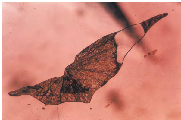
Figure 10 Crystallized melt inclusion in flux grown synthetic ruby. Note the deformed vapour bubble (transparent) and crystalline flux material.
