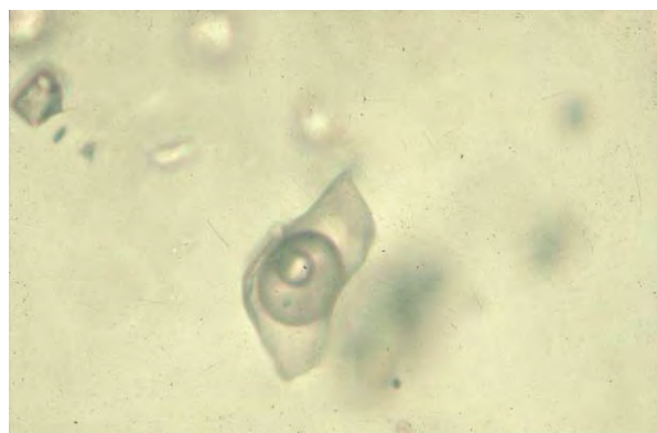
Figure 4 Three phase, liquid liquid gas (L + L + G) \text{CO}_2\text{-H}_2\text{O} inclusion with the characteristic ‘double bubble’ comprising an outer rim of liquid \text{CO}_2 enclosing a bubble of \text{CO}_2 gas.
