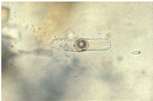
Figure 5 Aqueous inclusion containing two immiscible droplets of brown coloured oil in fluorite. Note the presence of a gas bubble in the larger oil droplet.
