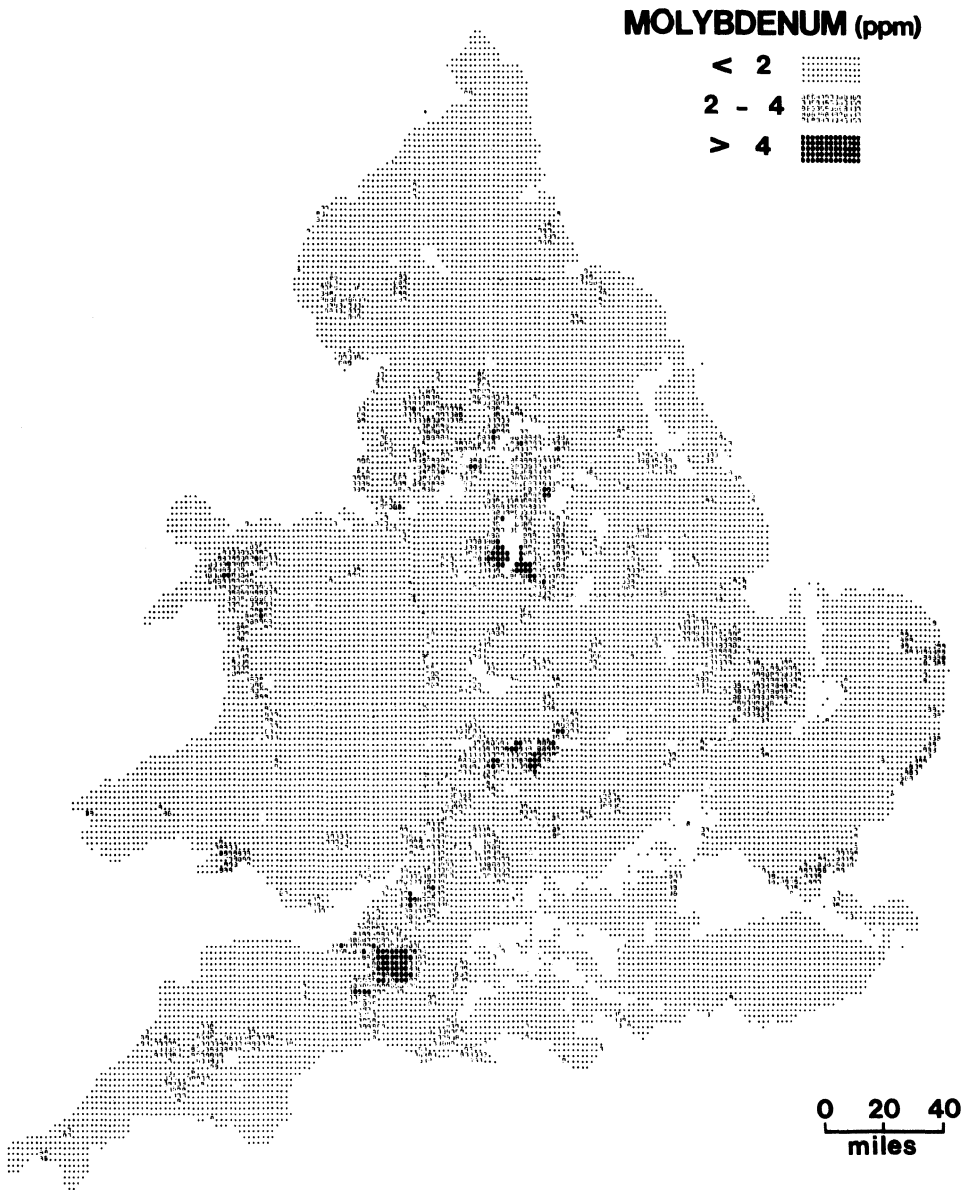
Fig. 1. Map showing distribution of molybdenum in stream sediments in England and Wales (compiled by the Applied Geochemistry Research Group as part of the Wolfson Geochemical Atlas of England and Wales, Webb et al., 1978).
