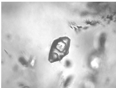
Figure 10. Photomicrograph showing a large isolated primary three-phase fluid inclusion (inclusion diameter = 25\text{ }\mu\text{m} ) in a pegmatitic segregation from the contact zone to garnet-amphibolites (retrograded eclogites) from the Münchberg Gneiss Complex in Germany. The inclusion contains—besides a liquid and a vapor-bubble—one unidentified solid phase, which did not dissolve during heating (for further explanation see text).
