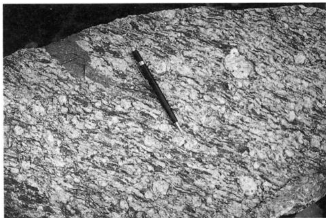
Figure 7. Fox Ridge granite (pluton G7) – strongly foliated, feldspar-augen, biotite granite. GSC 204394-H
