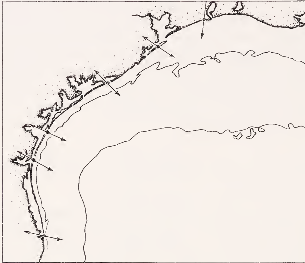
Fig. 74. Orientation of sand grains on the coast of Texas Bay. The arrows indicate orientation of long axes of sand grains. After J. R. Curray (1956).
