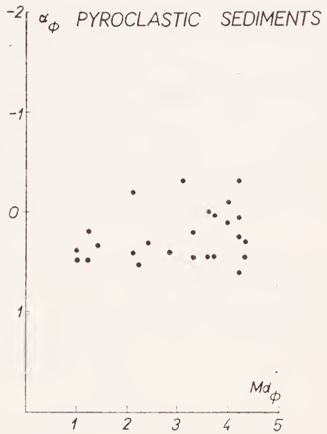
Fig. 42b. Grain-size parameters of pyroclastic sediments. Relation between Phi Median Diameter and Phi Skewness Measure.
