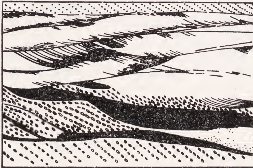
Fig. 53. Type of stratification of fluvio-glacial deposits. After L. N. Botvinkina (1962).
