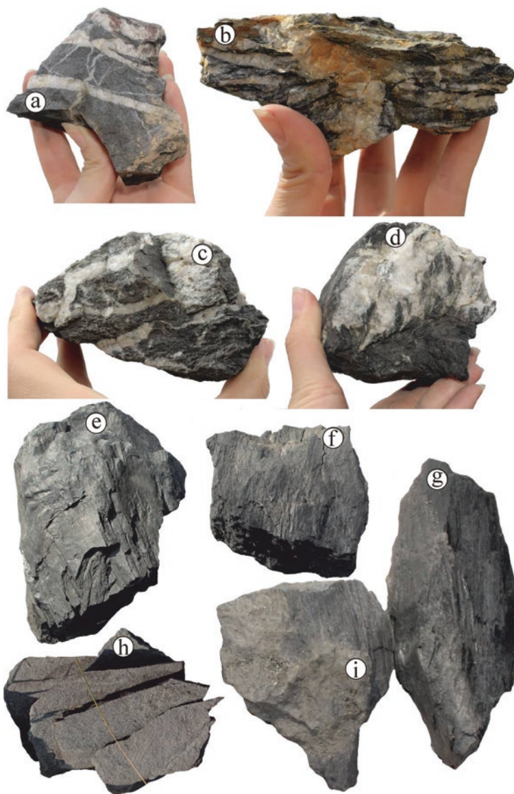
Samples: a, c, d – quartz-carbonaceous shales; b – ferruginous quartz-carbonaceous schist; e, f, g, h, i – carbonaceous shales.
