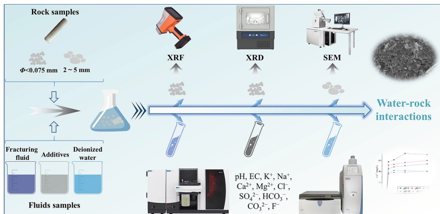
Fig. 5.1 Flow chart of the water–rock interaction experiment
