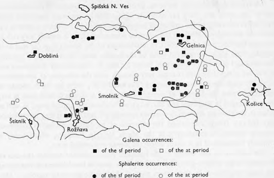
Fig. 7. The distribution of occurrences of sphalerite and galena of the sulphidic (sf) and stibnite period (at) in the Spiško-gemerské rudohorie Mts.
