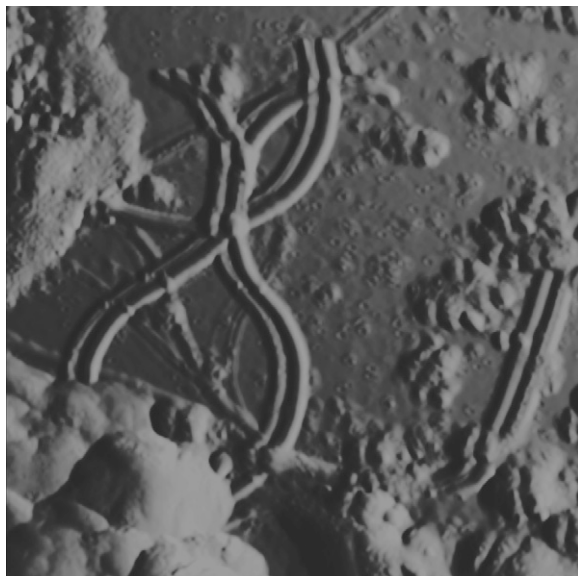
Fig. 11-9. Double tip artifact encountered on image of Pseudomonas mendocina following reaction with aluminous goethite. Several intertwined bacterial flagella are clearly doubled in this image.
