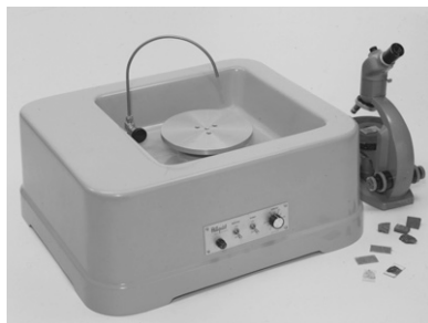
Fig. 7-6. Polishing machine used to smooth surfaces of chips that will be glued to glass slides. Depending on the model used, grinding materials can be powders or papers that are attached to the wheel. All grinding is done under a slurry, which can be water or a solvent. Photograph courtesy of Hillquist, Inc., Denver, CO.
