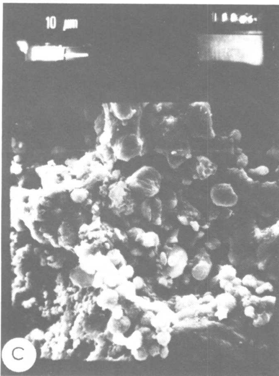
Fig. 10-9. Clay-rich material viewed under a scanning electron microscope (Hékinian and Fevrier, 1979). A. Green clay-rich material (CYP74-26-15-1) from Transform Fault "A" in the FAMOUS area (magnification \times 2400 ). B. Orange clay-rich material (CYP74-26-15) from Transform Fault "A" in the FAMOUS area (magnification \times 1300 ). C. Yellow clay-rich material (6243-12) from the Gulf of Aden (magnification \times 650 ). D. Green clay-rich material (Leg 54, 424-2-cc) from the Galapagos area (magnification \times 2500 ).
