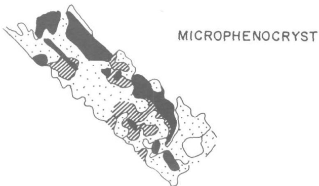
Fig. 9-6. Schematic representation traced after scanning electron microphotograph of plagioclase crystals showing progressive replacement of a calcic plagioclase by a more sodic plagioclase and by K-rich feldspar.
