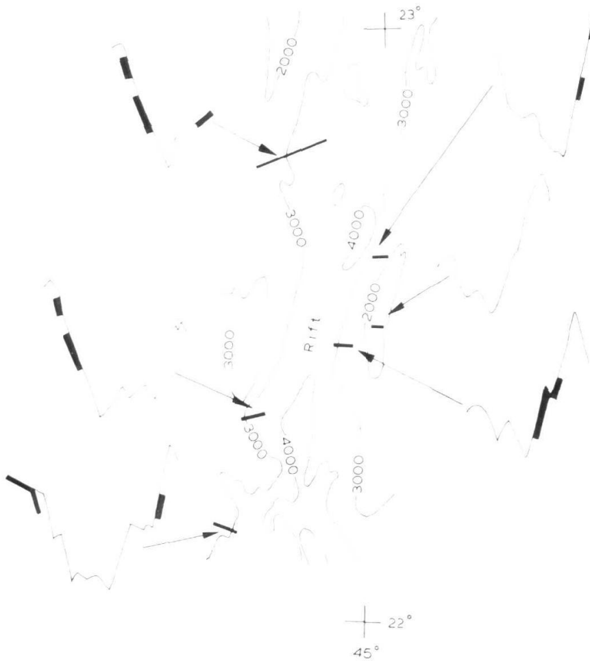
Fig. 2-3. Distribution of dredged samples in the Rift Valley near 22°N in the Atlantic Ocean after Van Andel and Bowin (1968). On the sides of the bathymetric map are the topographic profiles (vertical exaggeration about 12×) in corrected meters.
