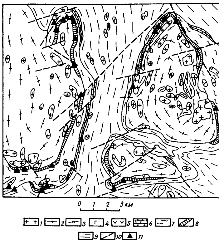
Fig. 44. Structural sketch map of the Sortavala ore region (after Ivashchenko, with the author's amendments). 1) late-orogenic granite; 2) granite–gneiss domes & migmatites; 3) early-orogenic granitoids; 4) metagabbro, quartz diorite; 5) metadolerite, metagabbro–dolerite, gabbro–amphibolite; 6–8) Sortavala Gp: 6) dolomitic marble, calciphyre, magnesian & apomagnesian lime skarns (u. carb. horizon), 7) amphibolite, amphibole–biotite & graphite schists with thin skarn layers, 8) magnesian & apomagnesian lime skarns; 9) quartz–biotite schist, migmatite, quartzite, quartzose sandstone (Ladoga Gp); 10) faults; 11) tungsten skarn ore occurrences.
