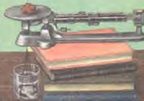
A balance used to measure specific gravity
