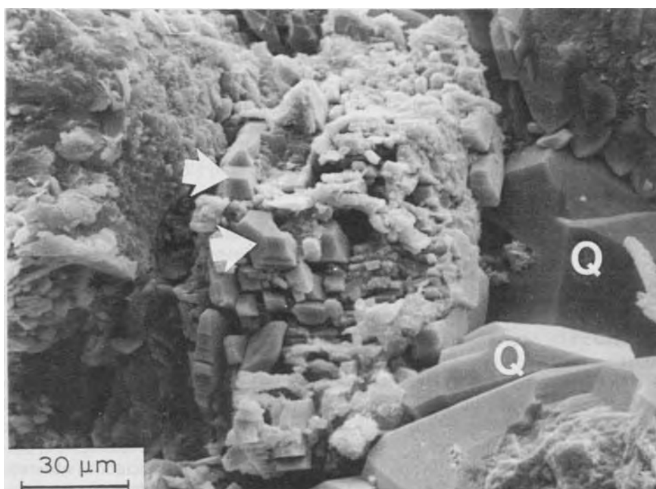
Fig. 1-24. Photomicrographs of albitization. Grain in center is a porous albitized plagioclase that has tiny euhedral overgrowths of albite (arrows) developed on parts of it. Q = quartz overgrowths. Miocene sandstone, Louisiana; depth = 6100 m.
