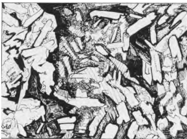
Fig. 4-16. Celadonite laths viewed under the SEM. Individual laths are about 3\ \mu\text{m} long. Glauconitic minerals never show this habit.
