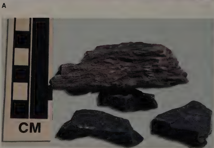
FIGURE 6.14 (A) An outcrop of shale from Hudson Valley in New York. Note how this fine-grained rock tends to split into very thin layers. (B) Shale pieces; note the very fine grain (scale in centimeters), very thin layers (laminations) on the edge of the large piece, and tendency to break into small, flat pieces (fissility). Photo A © John Buitenkant/Photo Researchers Inc.; Photo B by David McGeary
