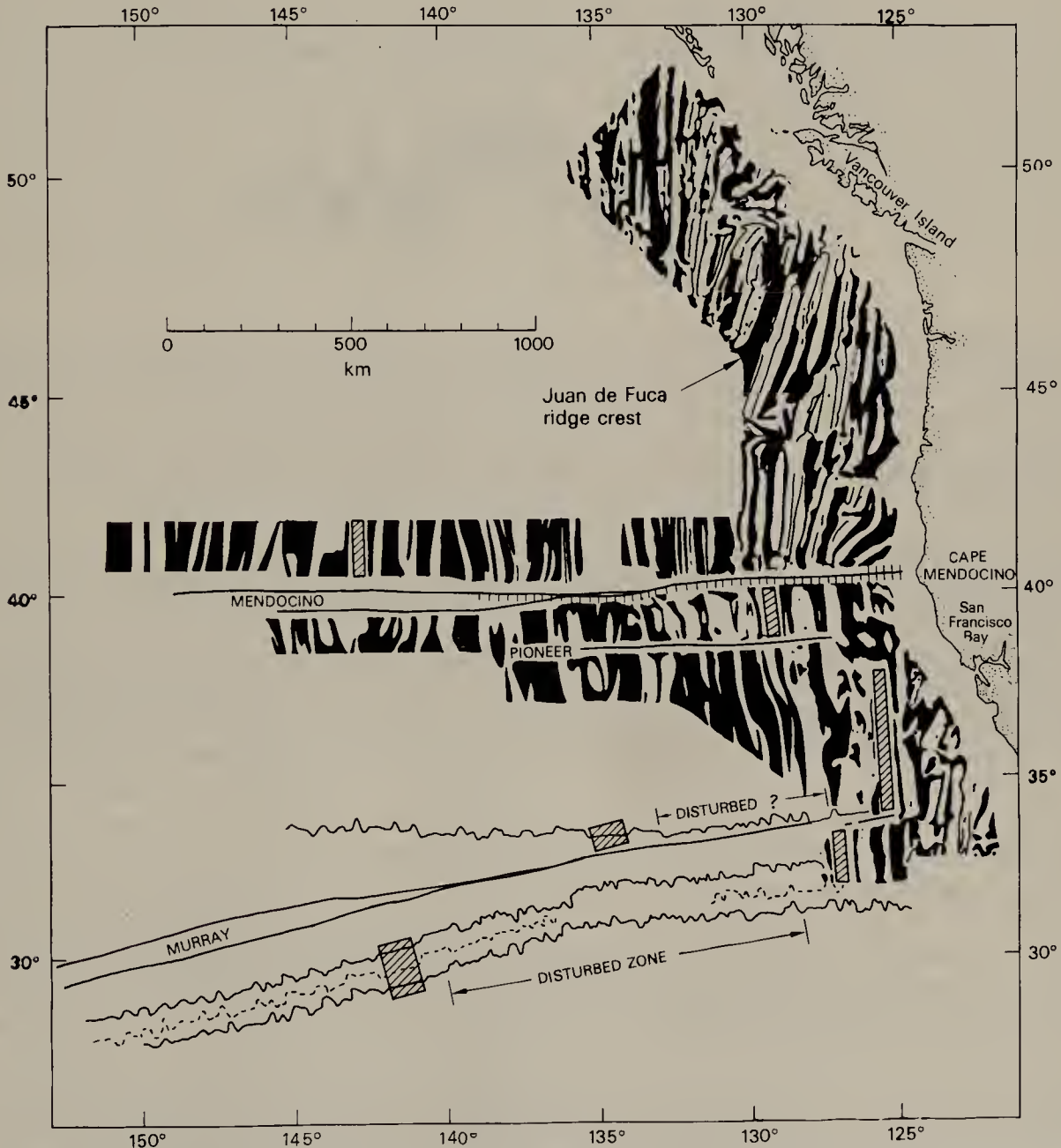
Fig. 3.7 Magnetic anomaly lineations off the west coast of North America. Positive anomalies are shown in black. Note the offset of the magnetic anomaly pattern at the fracture zones and the change in the amount of offset along the Murray fracture zone. After MENARD (1964), Marine geology of the Pacific , p. 46, McGraw-Hill.
