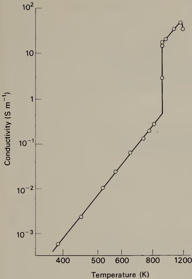
Fig. 4.27 Electrical conductivity of the iron-olivine fayalite ( \text{Fe}_2\text{SiO}_4 ) at 4380 MPa confining pressure as a function of temperature. Adapted from AKIMOTO and FUJISAWA (1965), J. geophys. Res. , 70 , 447.
