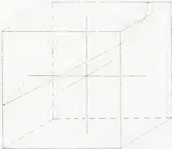
FIG. 72.—Block-diagram of the same plane on 'cabinet projection'.
