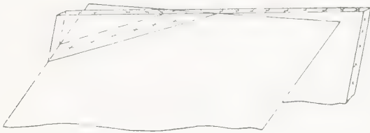
FIG. 15.—A vein intersecting a dipping bedding-plane.
