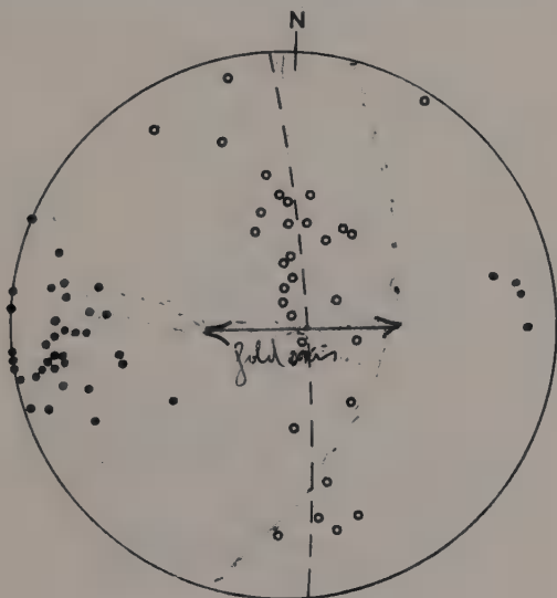
FIG. 80.—Stereogram of normals to schistosity and poles of lineations, Start area, S. Devon.
